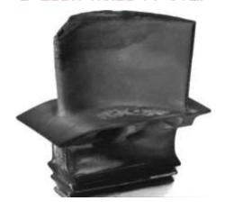
Fig2: View of a failed blade
