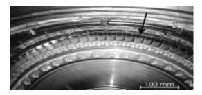
Fig6: Uneven clearance between blade tip and rotor lining
