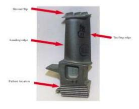
Fig1. Blade failure location
